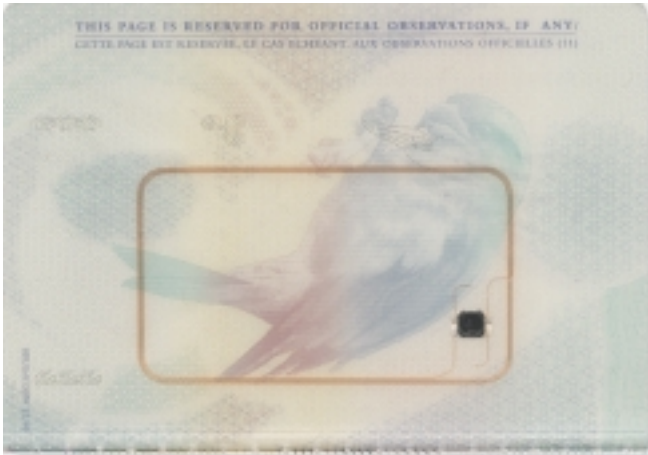
Figure 5-14: View of a proximity chip, applied in an British passport. (Courtesy of National Criminal Intelligence Service, the Netherlands.)
