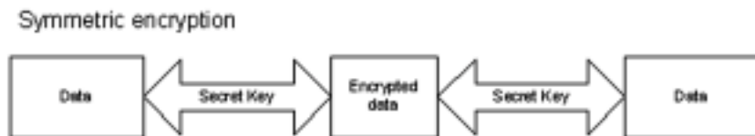
Figure 8-2: In symmetric encryption, a single, shared secret key is used for encrypting and decrypting data. Both the encrypting and decrypting parties can use the same key and perform the same actions.
