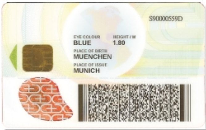
Figure 5-11: View of an Two Dimensional (2D) Barcode applied on a sample card. (Courtesy of Giesecke & Devrient, Munich, Germany.)
