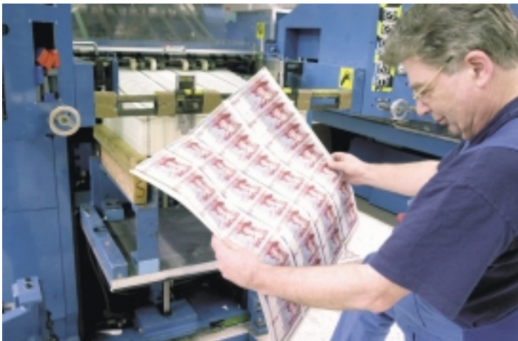
Figure 1-7: Product control at the press (Courtesy of Setec Oy of Finland)
