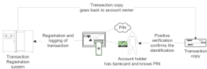
Figure 8-1: The account holder has a bank card and knows his PIN, enabling him to withdraw cash from a cash dispenser. The transaction is logged and a bank statement is sent to the account holder. If the account holder accepts the transaction, positive verification is confirmed.
