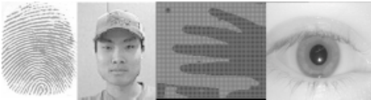
Figure 7-1: Fingerprint, face, hand and iris system sensor images. (Courtesy of Jim Wayman, San José, United States of America)
