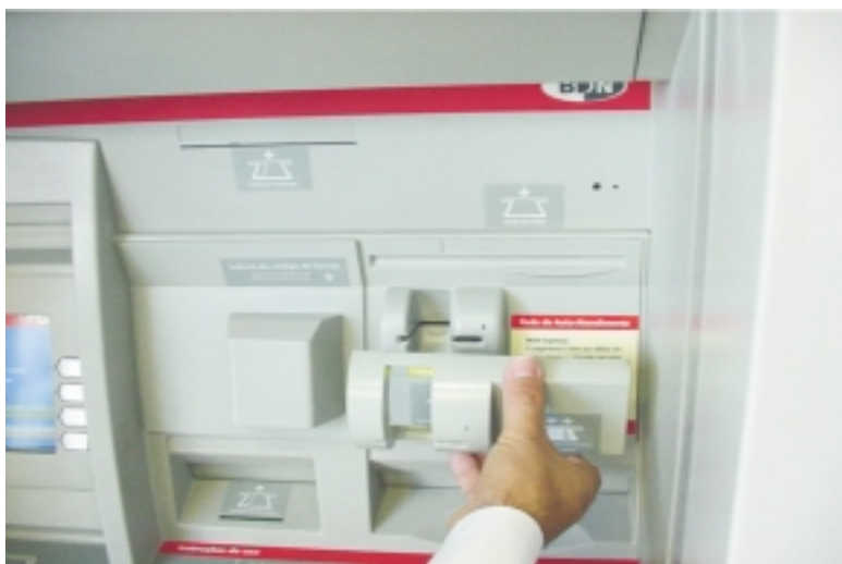
Figure 5-10: View of an skimming device placed up front an Automated Teller Machine (ATM). This skimming device is copying and storing the information of the magnetic stripe of a payment card.
