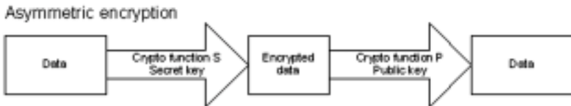
Figure 8-4: With asymmetric encryption, data that has been encrypted with the secret key (only known to the holder) can only be decrypted with the public key.
