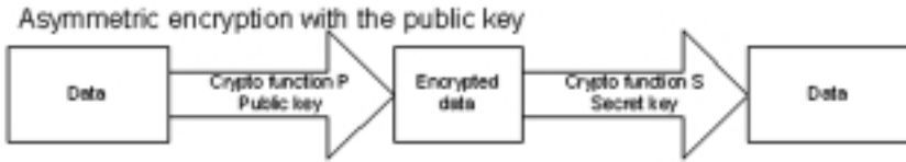
Figure 8-3: With asymmetric encryption, data that has been encrypted with the public key can only be decrypted with the secret key, which is only known to the holder of the secret key.
