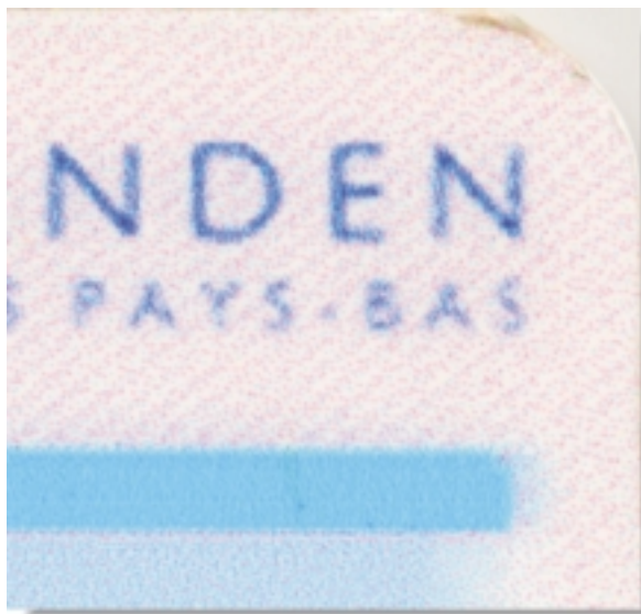
Figure 5-6: View of inkjet printing applied onto an Dutch counterfeit Identity card. The characteristics of the coloured dots are clearly visible. (Courtesy of Sdu Identification, Haarlem, the Netherlands.)
